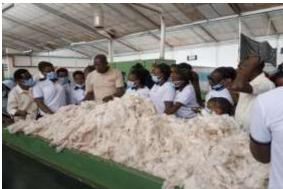
Above they are seeing the raw cotton after initial sorting and cleaning, being prepared for the spinning stage. An instructor is explaining the many cleaning steps after cotton is picked.
